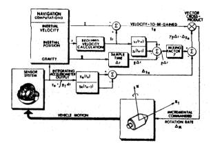
Figure 4. Velocity-to-be-gained steering
