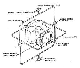
Figure 5. IMU schematic diagram
