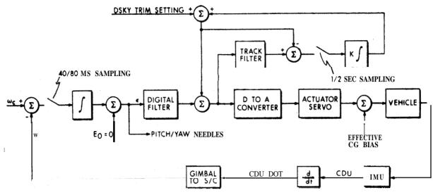
Figure 8. Powered flight autopilot
