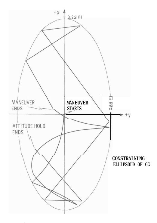
Fig. 4. <sup>2</sup> Propellant Motion Due to Attitude Maneuver
