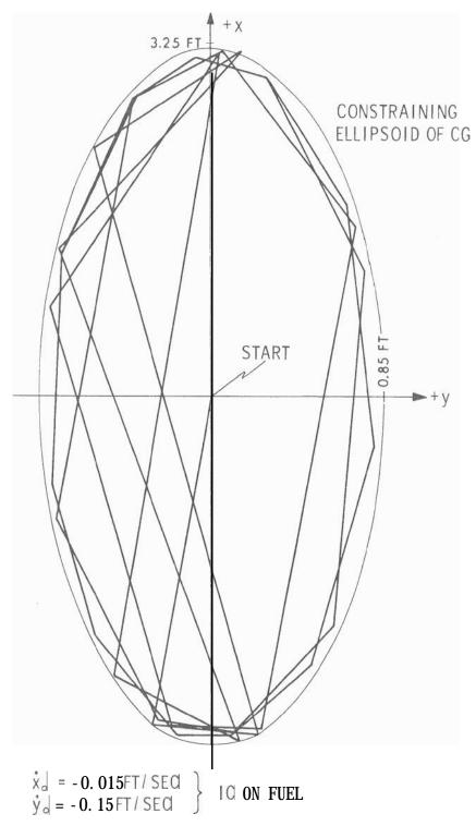
Fig. 4. 3 Propellant Motion in Attitude Hold
