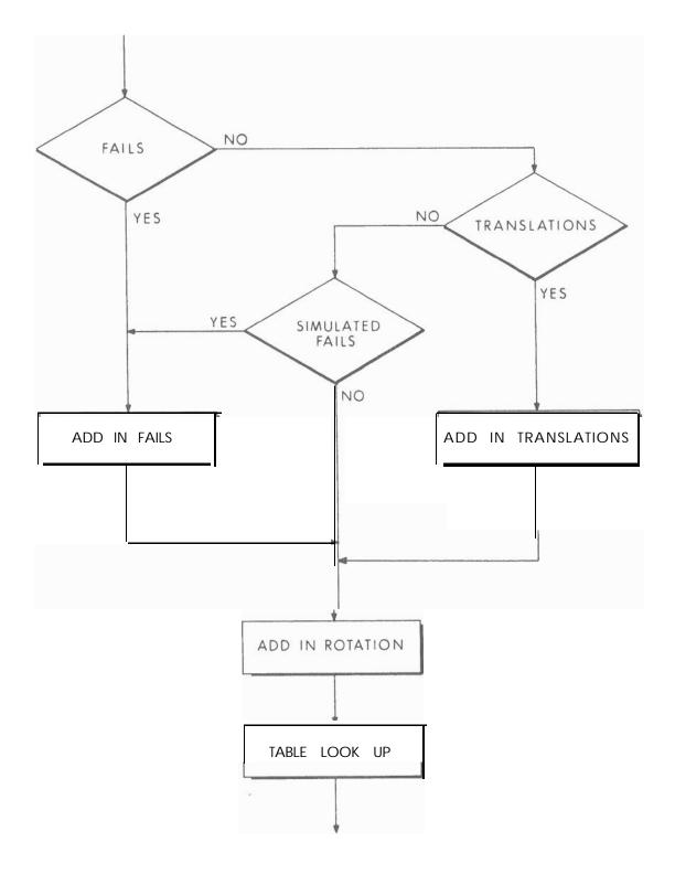
Fig. 3.2 Logic for Rotation Quads
