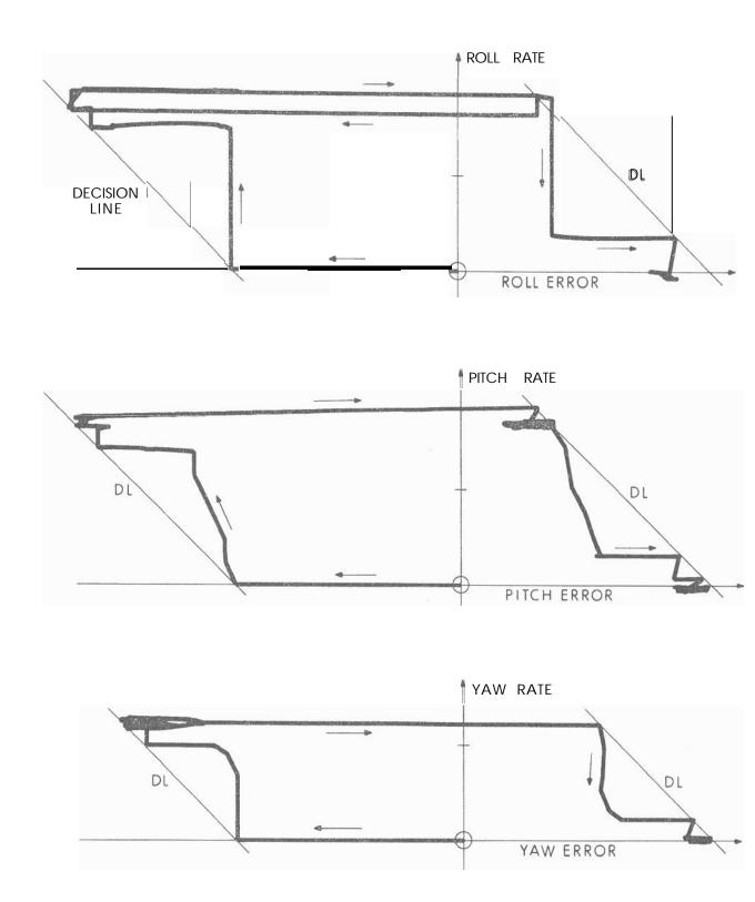
Fig. 4.1 Phase Planes for 3-Axis Maneuver
