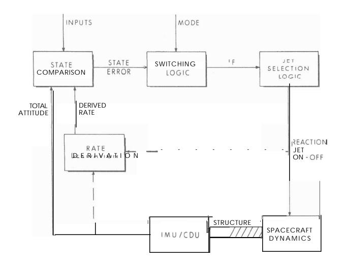
Fig. 2. 1 Block Diagram of Autopilot
