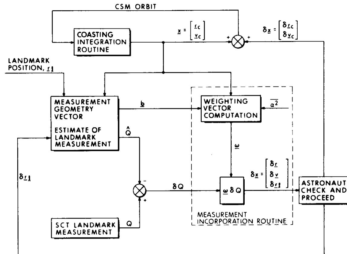
Fig. 2.1-1 Simplified Orbit Navigation Functional Diagram
