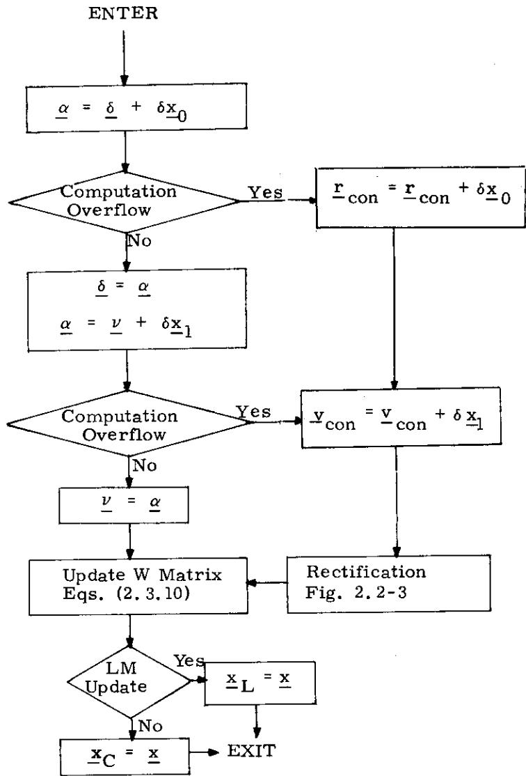
Fig. 2.3-2 INCORP2 Subroutine Logic Diagram
