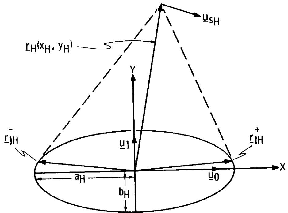
Figure 2.6-2 Geometry of Star-Horizon Measurement
