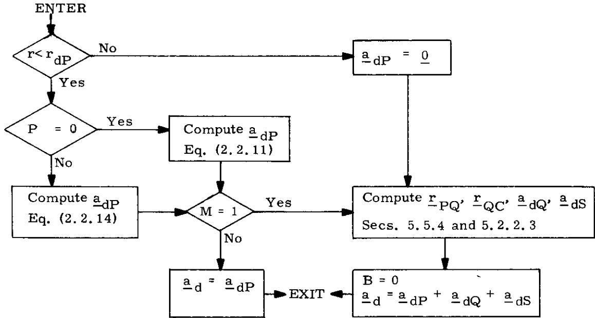
Figure 2.2-4 Disturbing Acceleration Selection Logic Diagram
