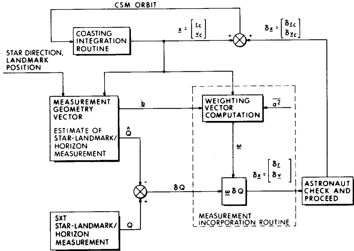
Fig. 2.1-3 Simplified Cislunar-Midcourse Navigation Functional Diagram
