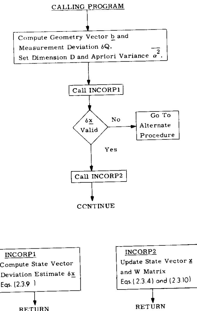
Fig. 2.3-1 Measurement Incorporation Procedure
