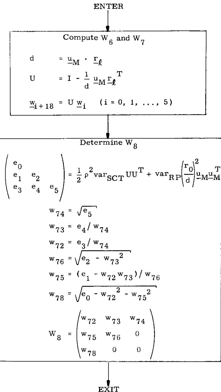
Fig. 2.4-3 W Matrix Initialization for Unknown Landmark
