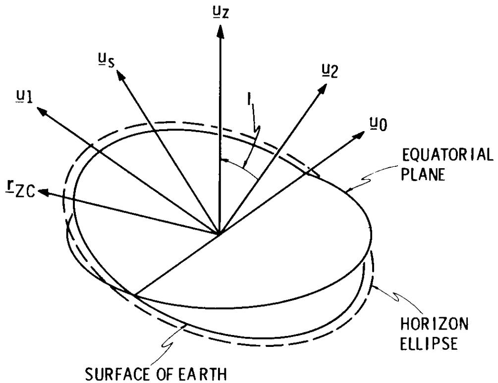
Figure 2.6-1 Definition of Horizon Coordinate System
