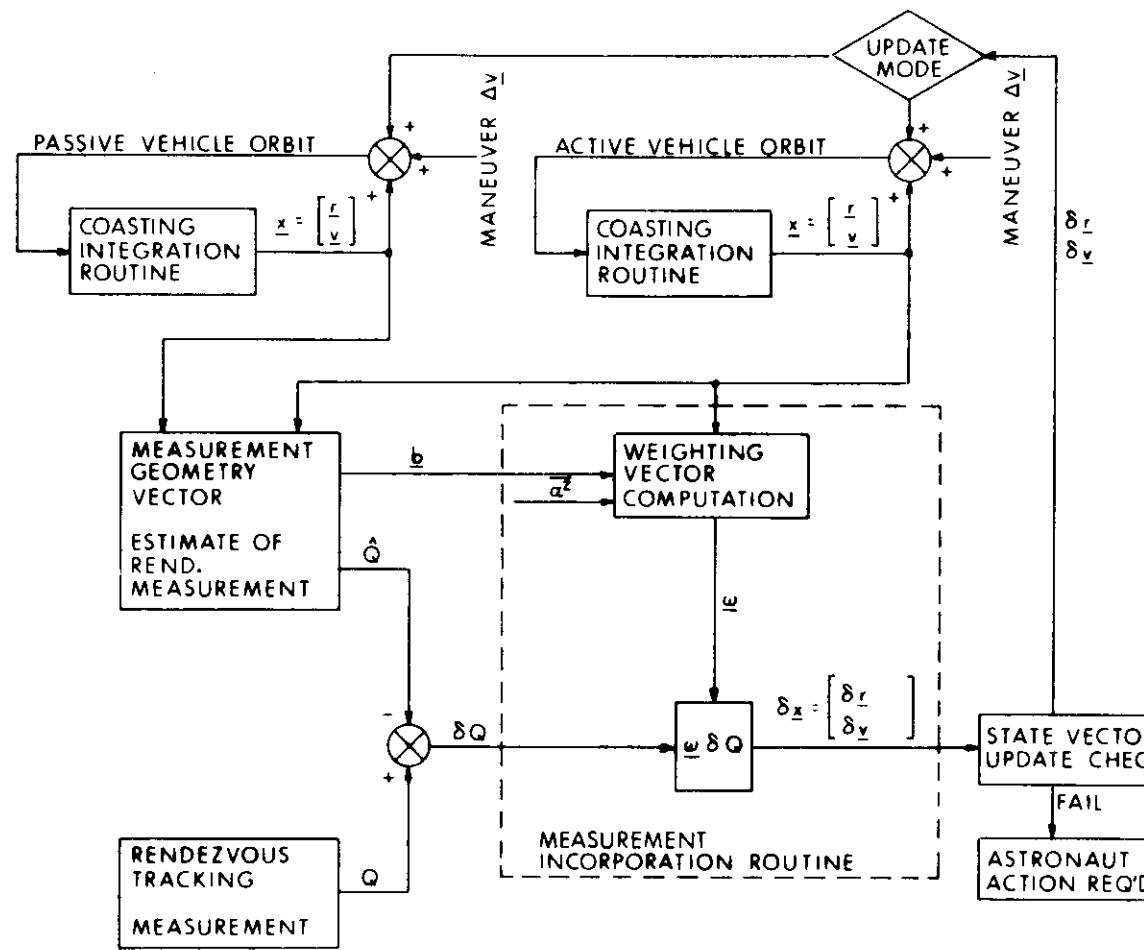
Fig. 2.1-2 Simplified CMC Rendezvous Navigation Functional Diagram
