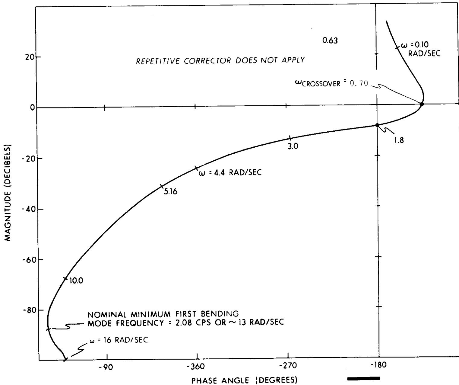
Fig. 3.3.4 Gain-Phase Plot of CSM/LM Control System
