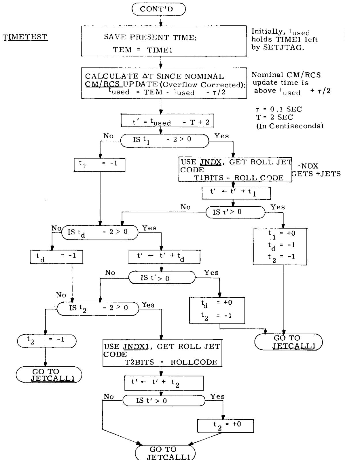
Fig. 3.4.37 Roll DAP - Time Interval Processing.
