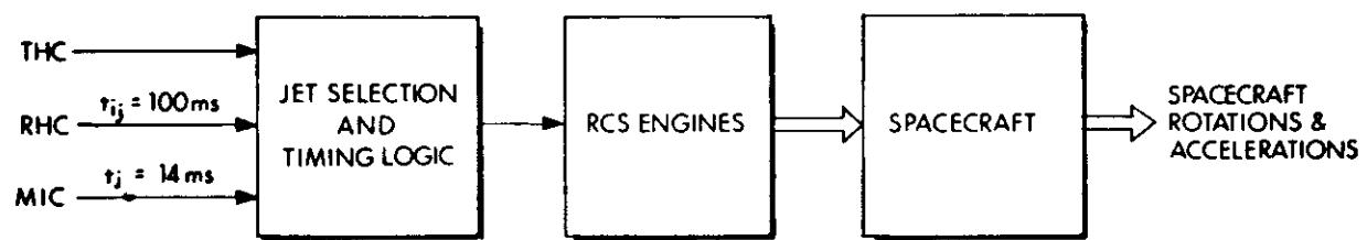
Fig. 3.2.5 PGNCS RCS Attitude Control Free Acceleration Control
