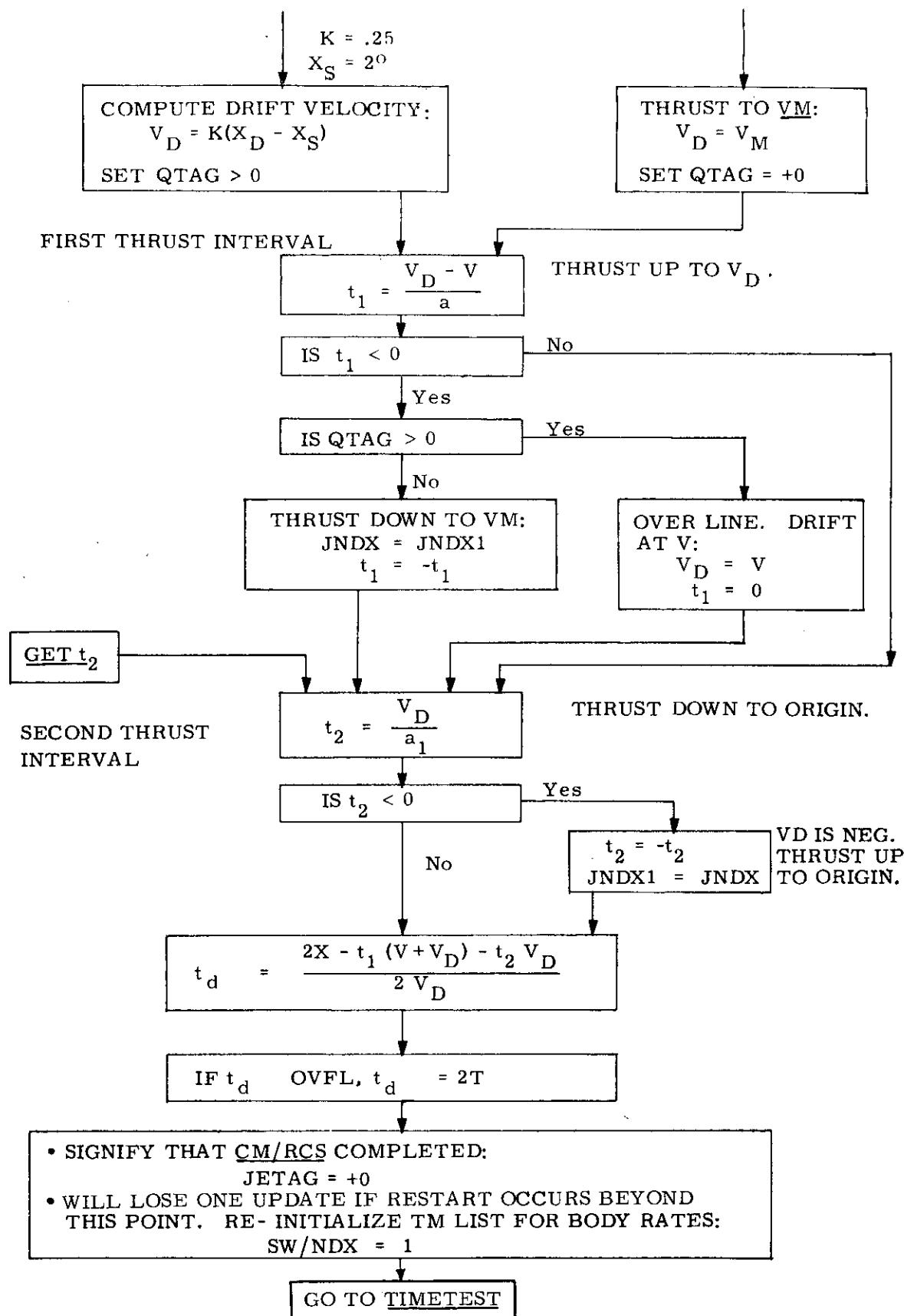
Fig. 3.4.36 Dual Gain Roll DAP - Time Calculations.
