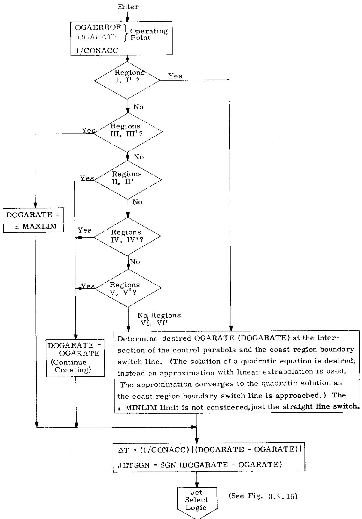
Fig. 3.3.15 TVC ROLL DAP Phase Switching Logic
