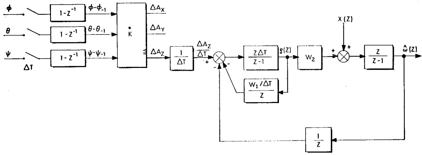
Fig. 3.2.6 CSM-RCS Digital Autopilot Rate Filter
