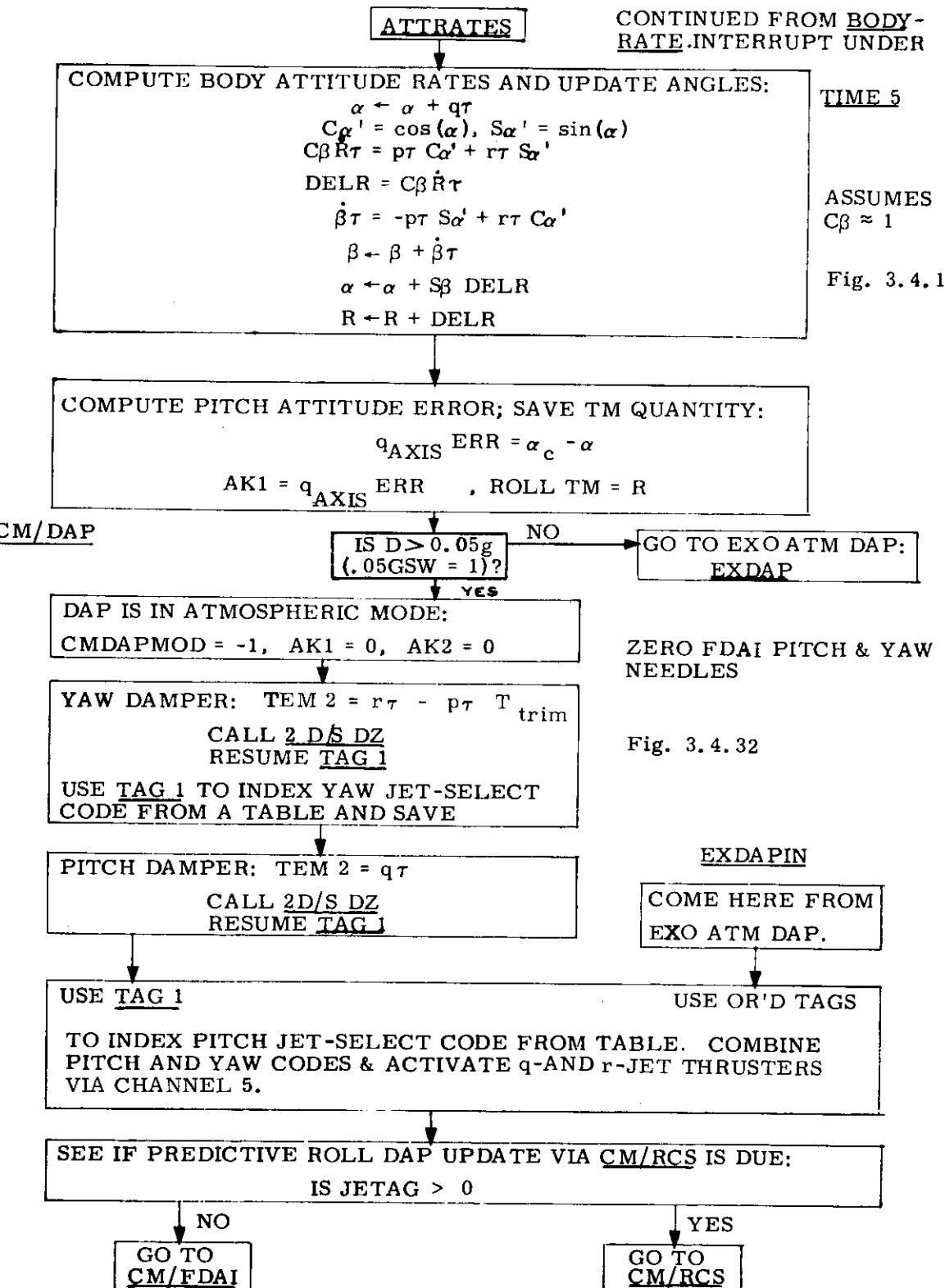
Fig. 3.4.30 CM Attitude Angles; Pitch and Yaw Dampers.
