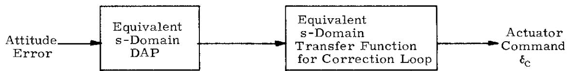
Fig. 3.3.11 Equivalent s-Domain Transfer Function of Thrust-misalignment Estimator Loop
