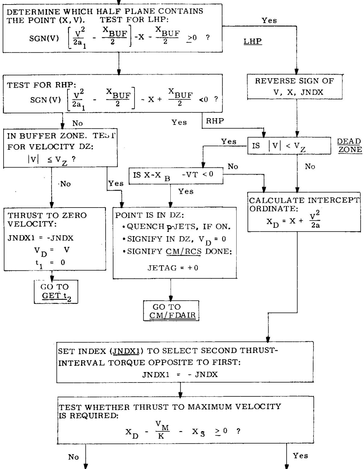
Fig. 3.4.35 Dual Gain Roll DAP - Initial Logic.
