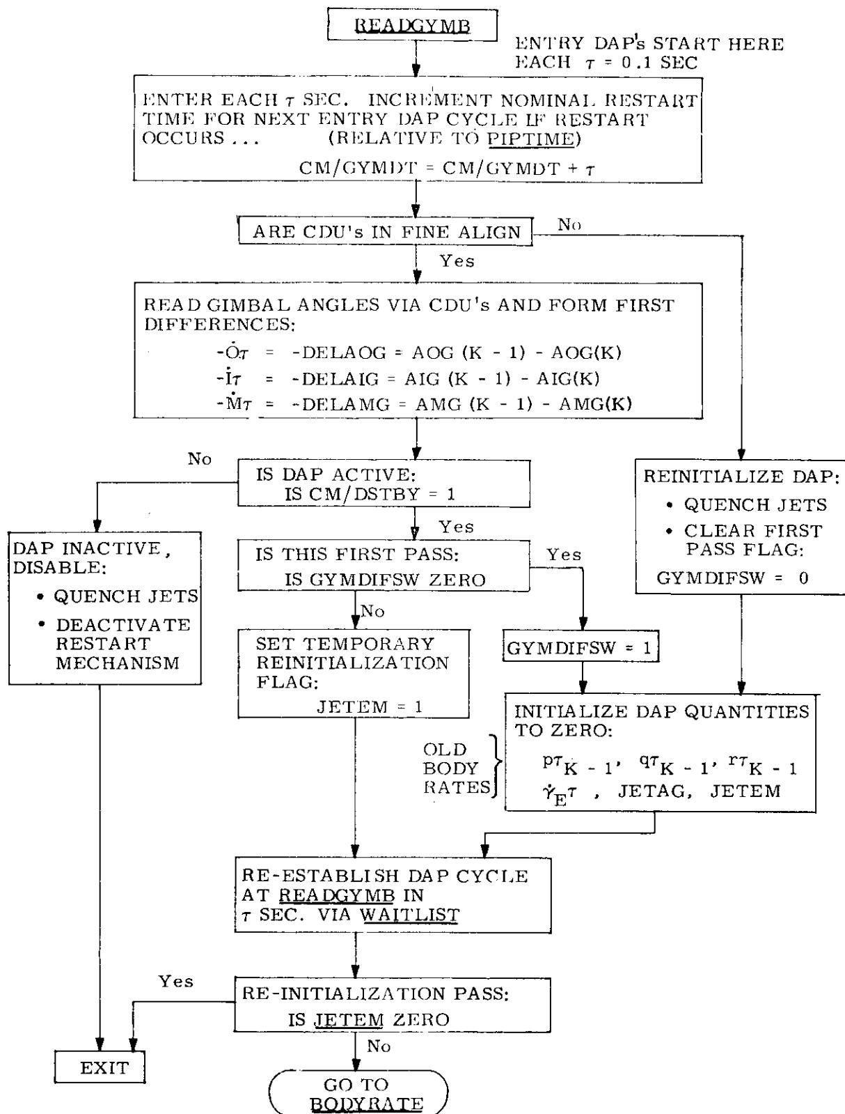
Fig. 3.4.28 Gimbal Angle Rates & Body Rate Initialization.
