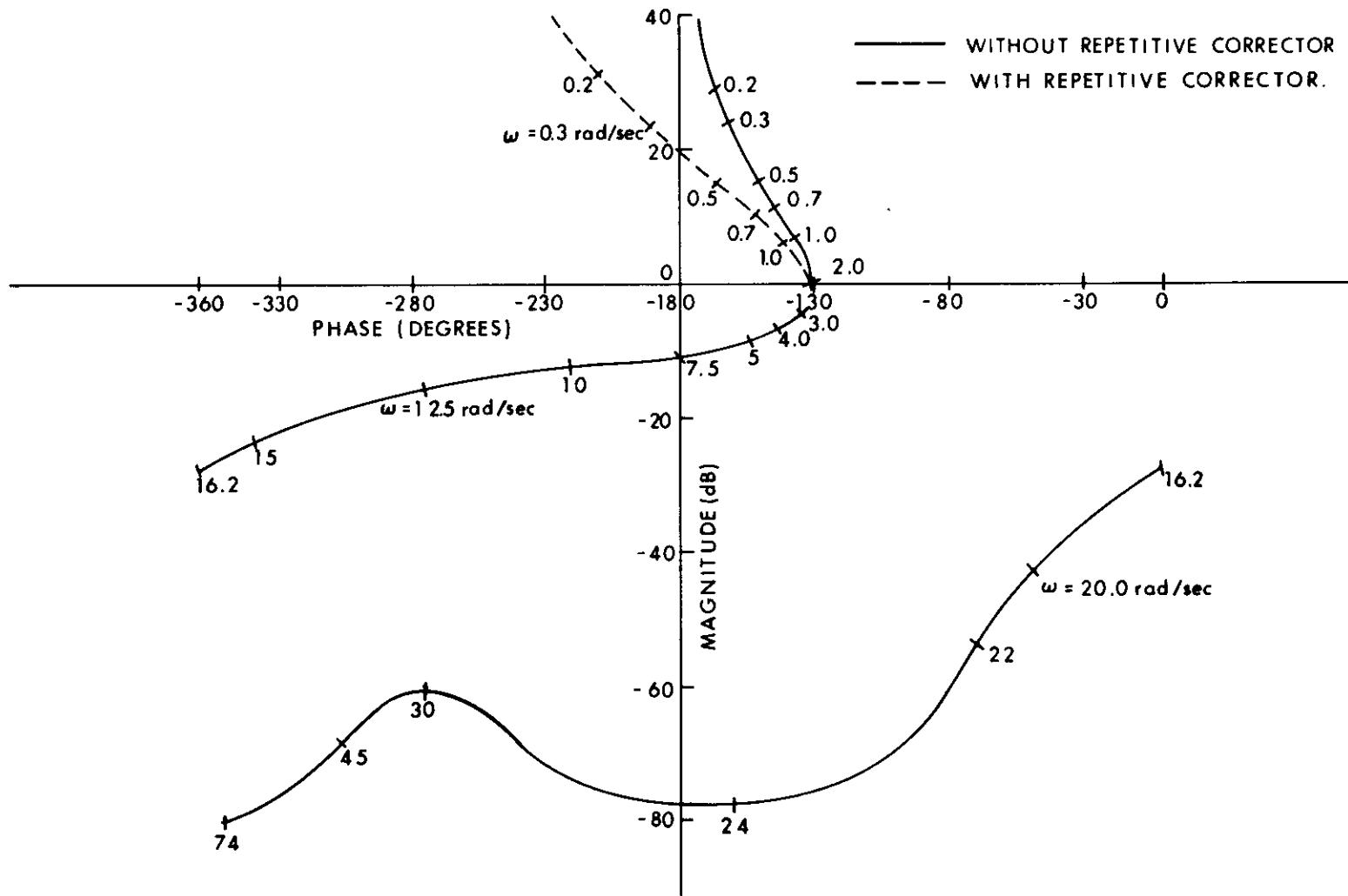
Fig. 3.3.5 Gain versus Phase Plot of CSM Control System
