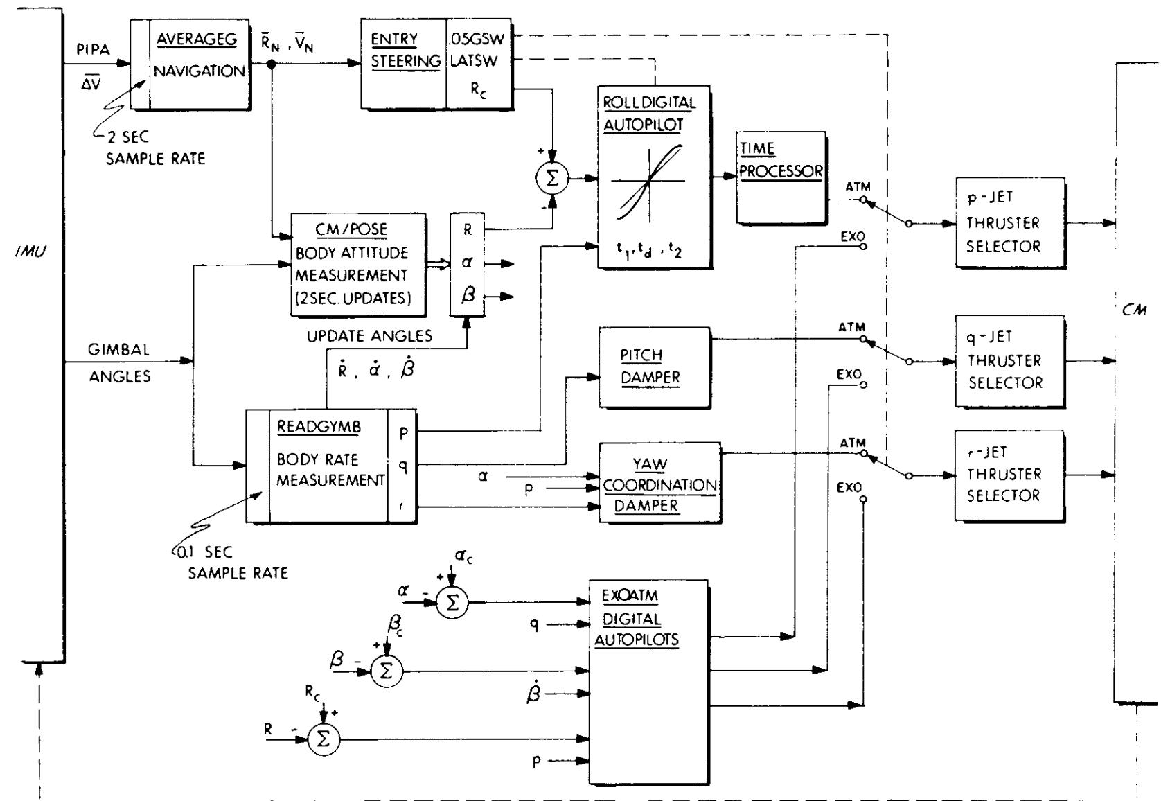
Fig. 3.4.2 Block Diagram of ENTRY Digital Autopilot
