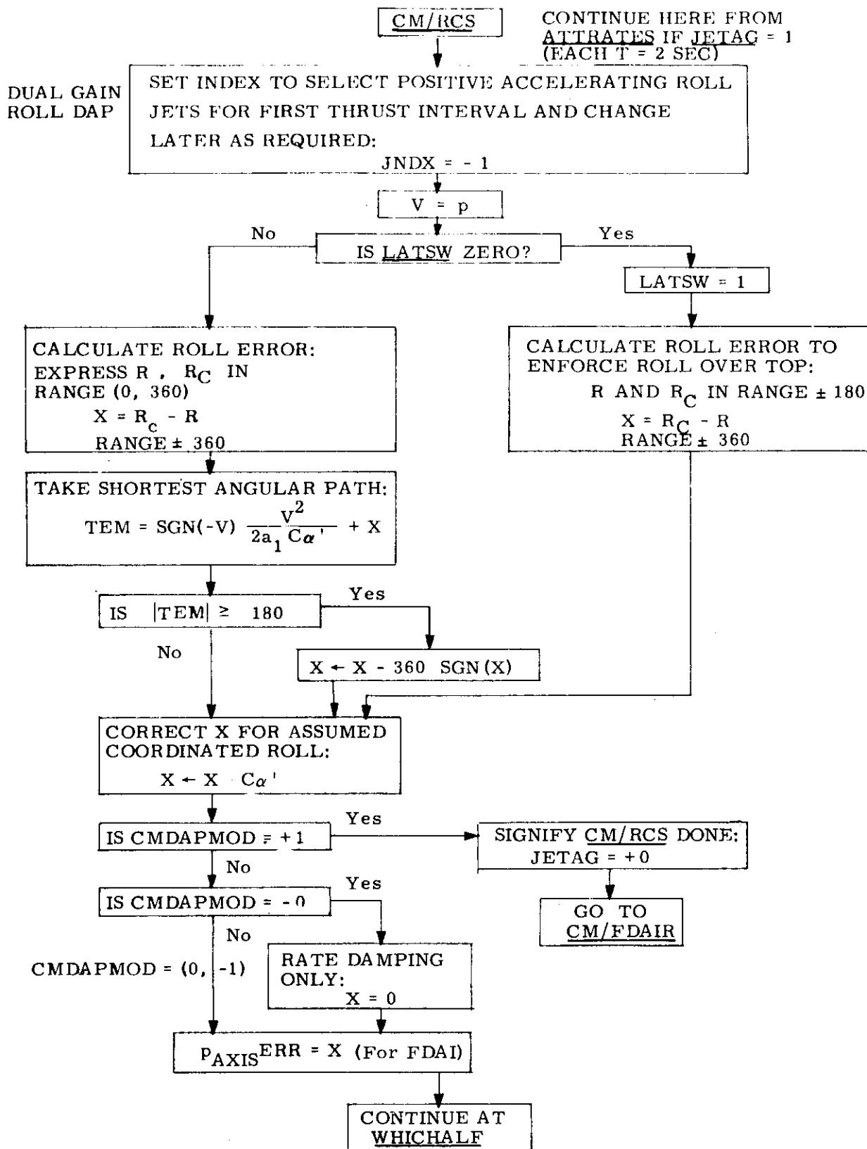
Fig. 3.4.34 Dual Gain Roll DAP - Error Calculation.
