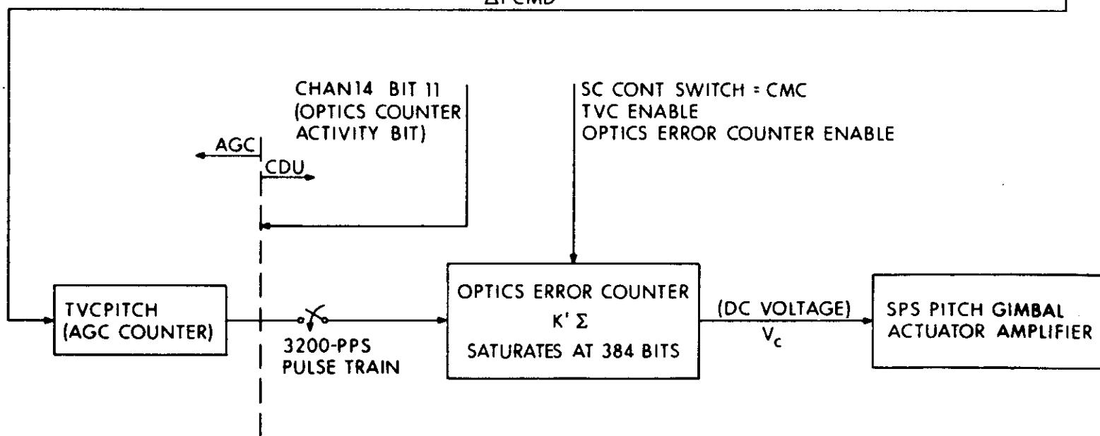
Fig. 3.3.21 TVC Actuator Command Interface: Pitch Channel
