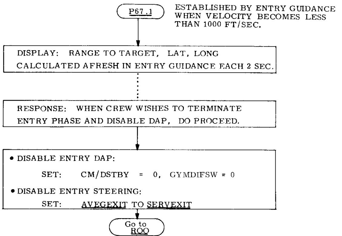
Fig. 3.4.9 Termination of Entry Control (P60s)
