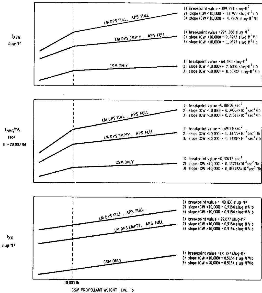
Fig. 3.3.8 Sketch of Curves Used by Program
