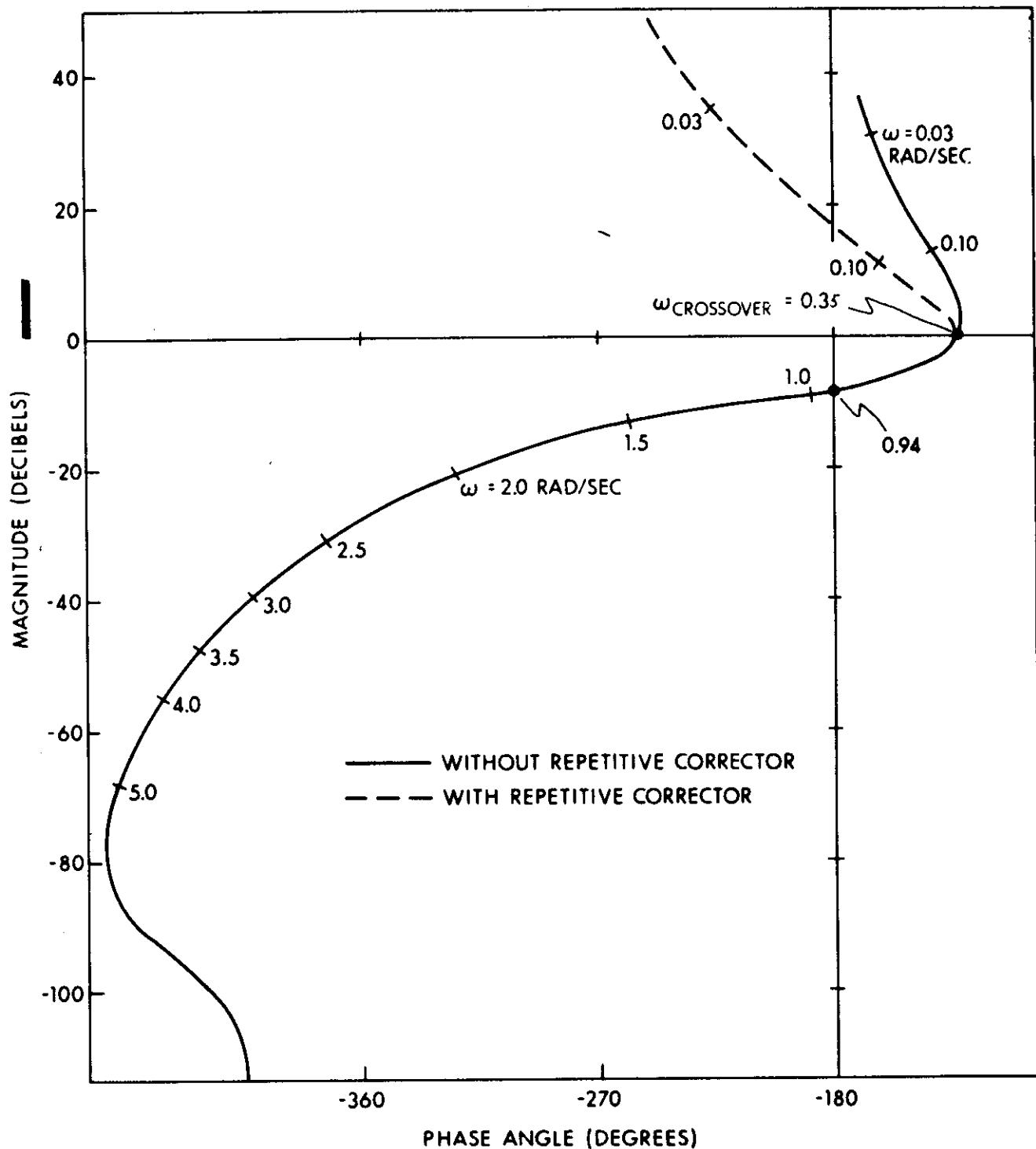
Fig. 3.3.3 Gain-Phase Plot of CSM/LM Control System
