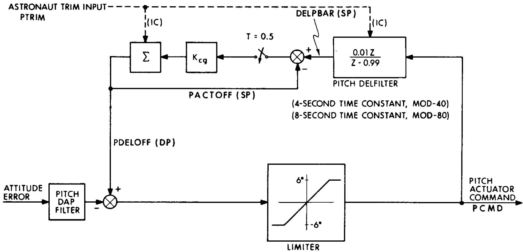
Fig. 3.3-10 Block Diagram of Pitch-Thrust Misalignment Correction Loop
