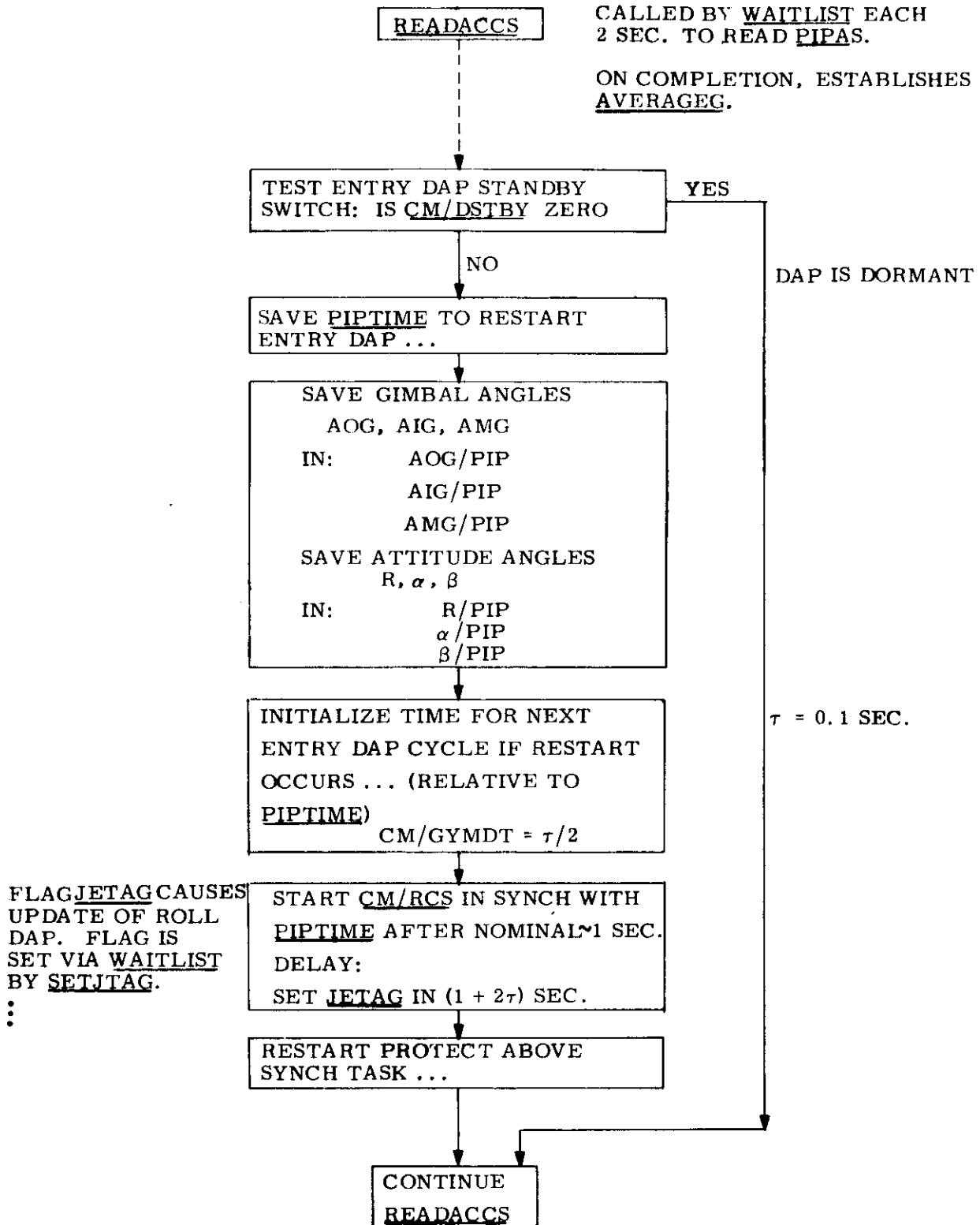
Fig. 3.4.16 Initialization of Body Attitude Calculation (CM/POSE).
