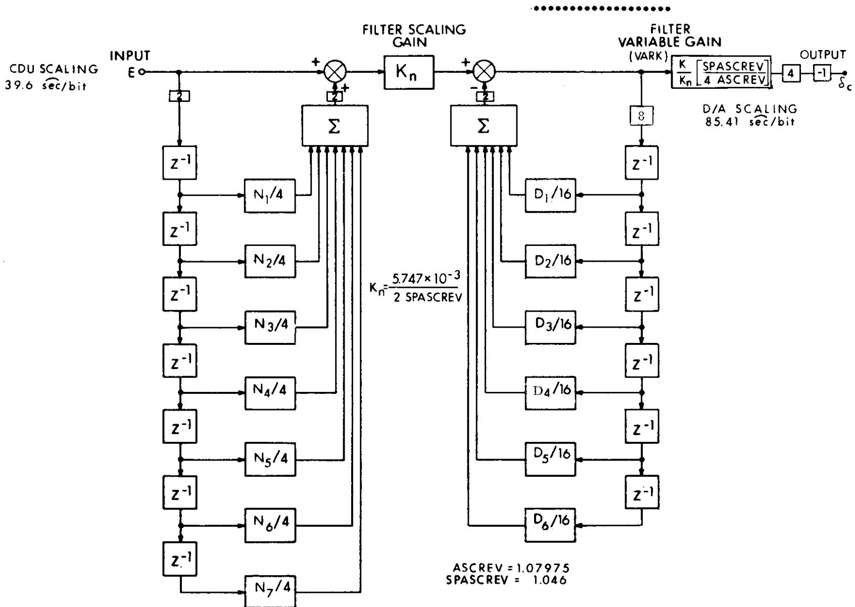
**Fig. 3.3.6 CSM/LM Filter**
