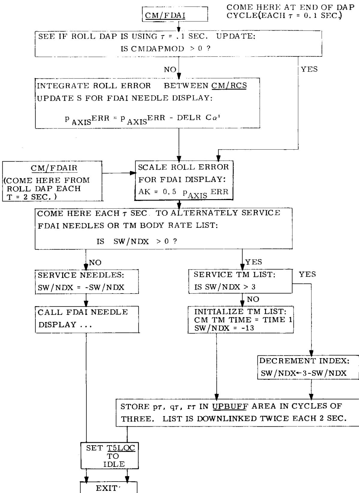
Fig. 3.4.39 Entry DAP Display and Telemetering Interface.
