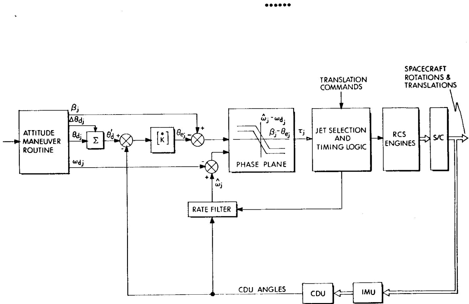
Fig. 3.2.3 PGNCS RCS Automatic Control Logic
