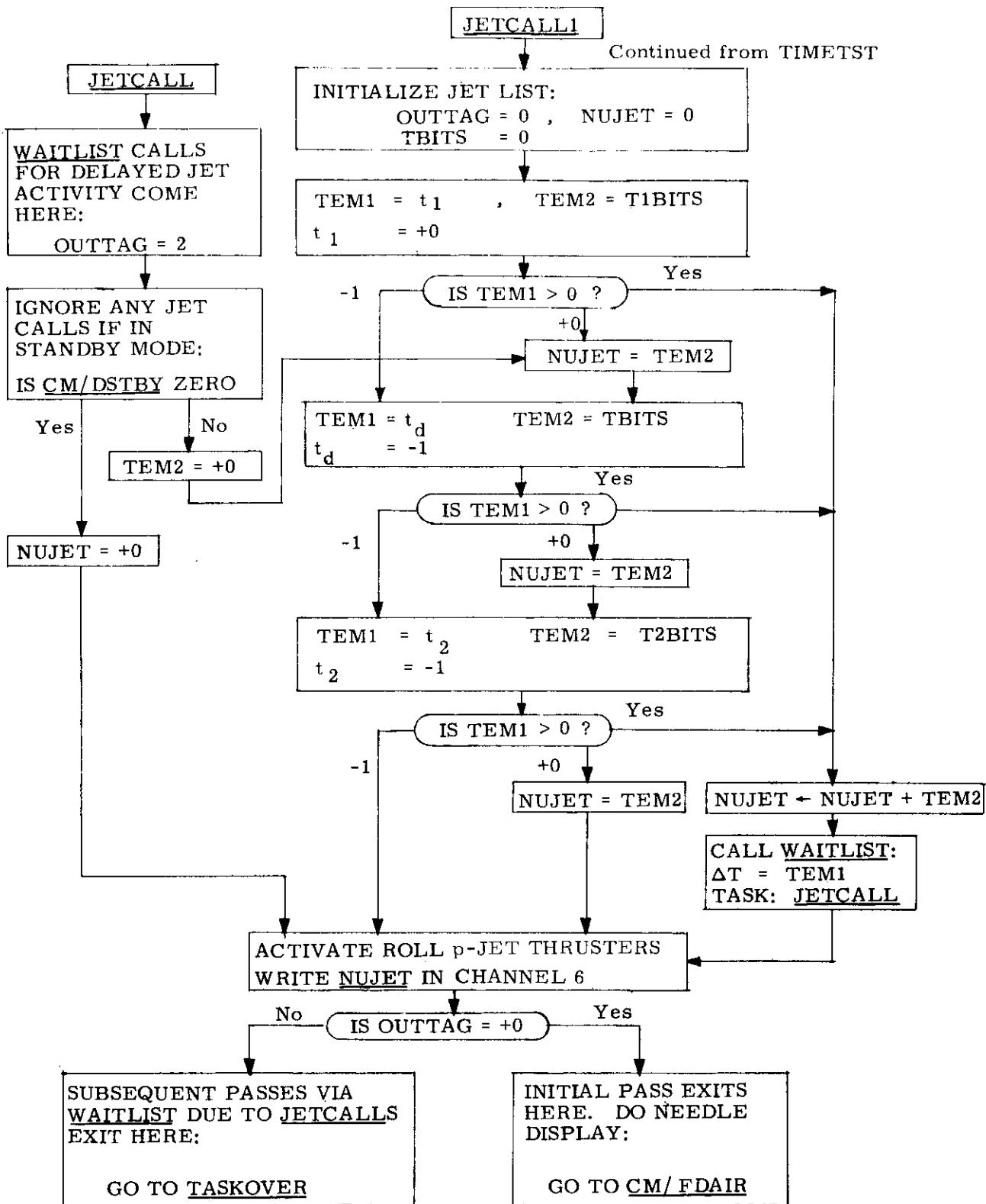
Fig. 3.4.38 Roll DAP - Time Interval Execution Logic.
