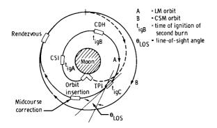
Figure 3. - Coelliptic rendezvous flight profile.
