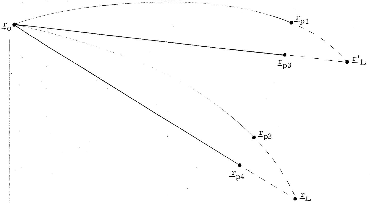
$$t_p = t + \sqrt{\frac{a^3}{\mu}} (E - e \sin E) + 16 \times 10^{-10} r_o (r_p - r'_p)$$
