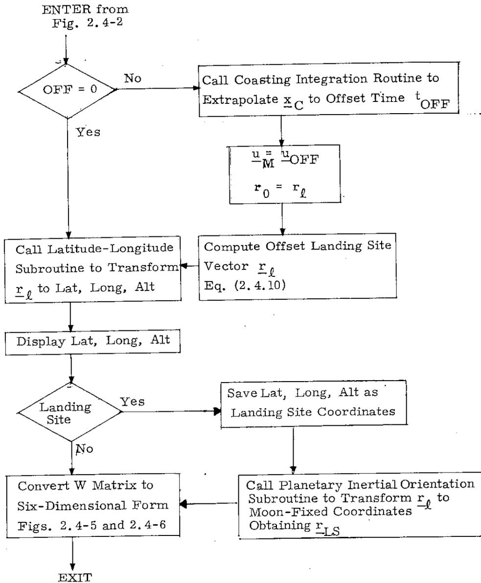
Fig. 2.4-4 Orbit Navigation Routine Termination
