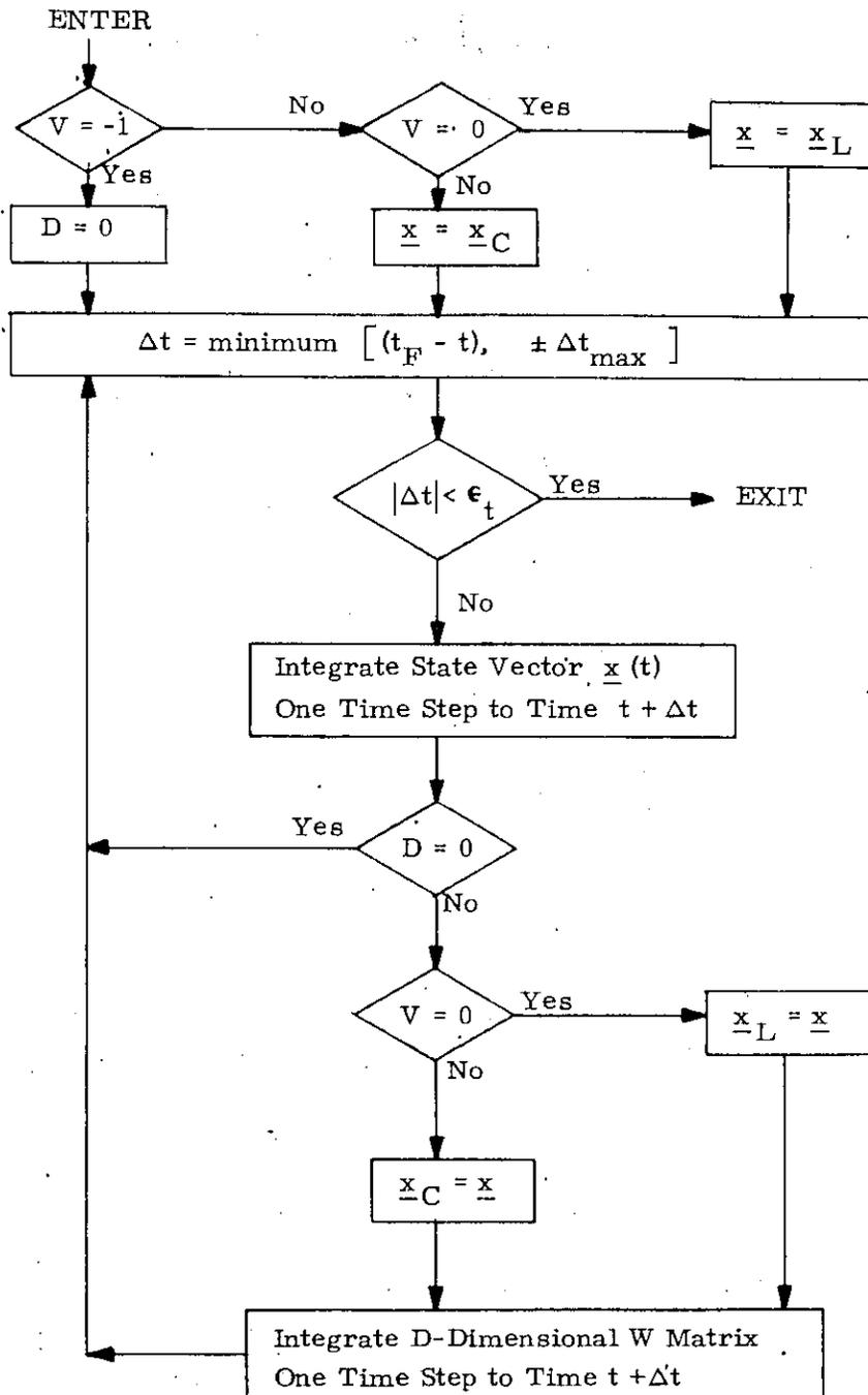
Figure 2.2-1 Simplified Coasting Integration Routine Logic Diagram
