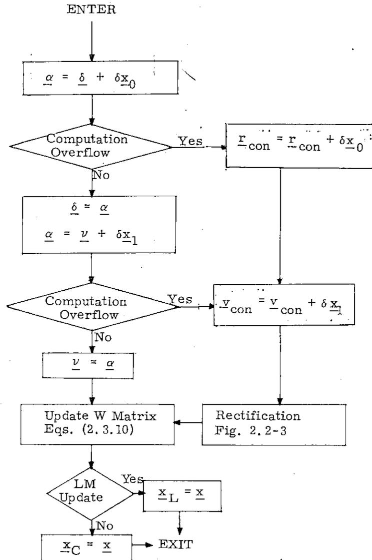
Fig. 2.3-2 INCORP2 Subroutine Logic Diagram
