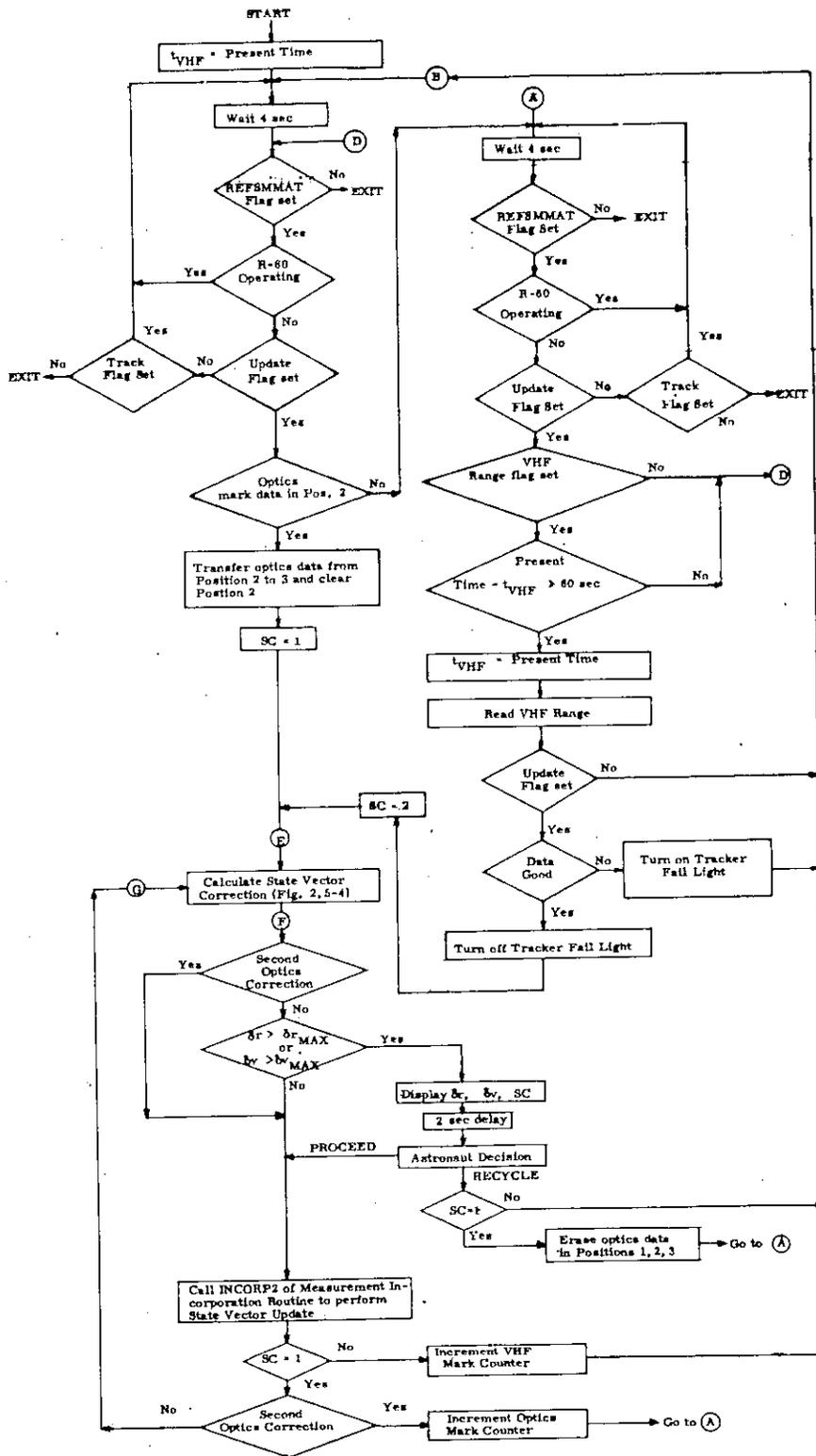
Figure 2.5-3 Rendezvous Tracking Data Processing
