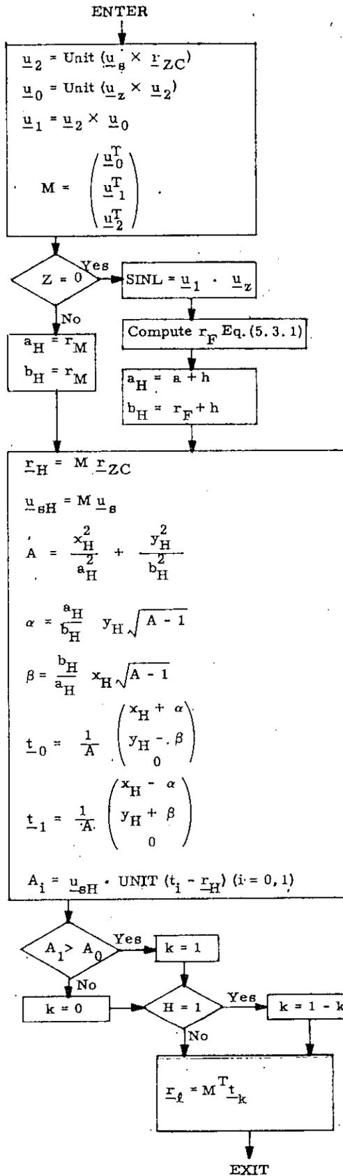
Figure 2.6-5 Horizon Vector Determination Logic Diagram
