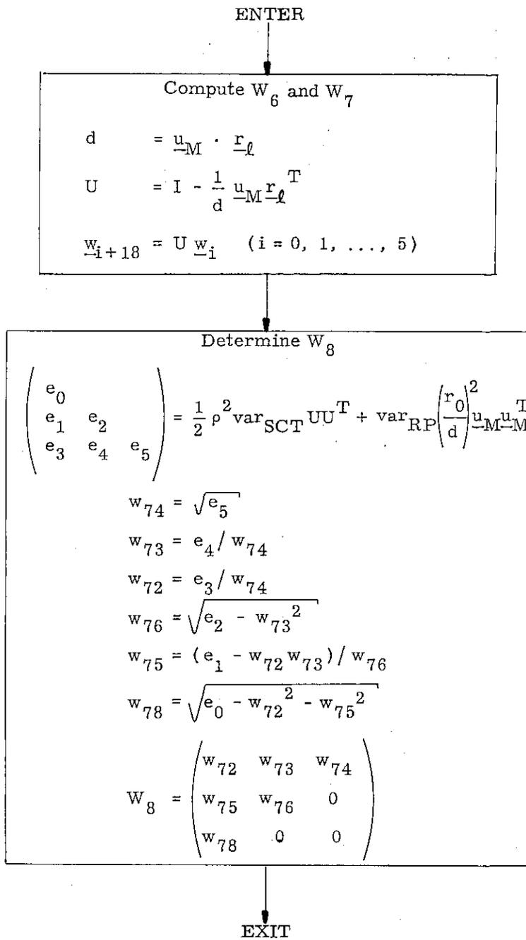
Fig. 2.4-3 W Matrix Initialization for Unknown Landmark
