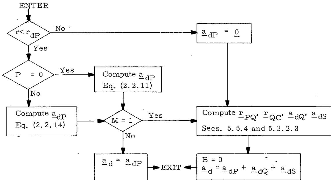
Figure 2.2-4 Disturbing Acceleration Selection Logic Diagram
