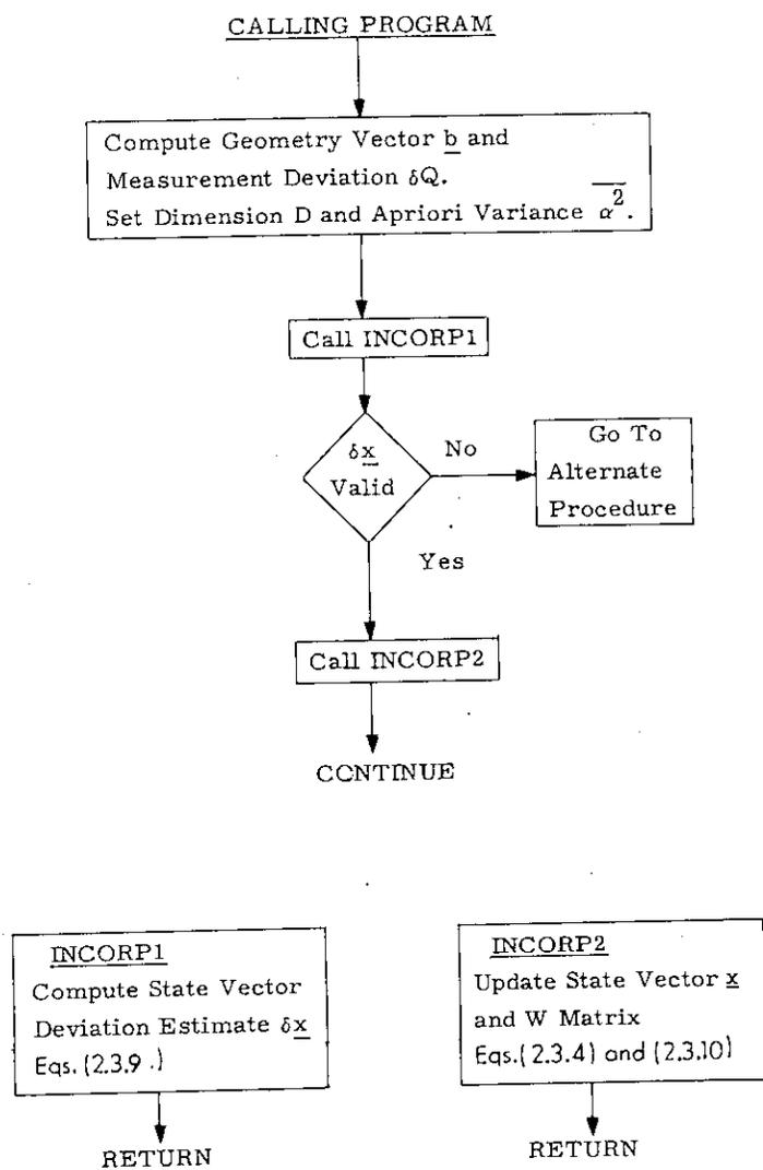
Fig. 2.3-1 Measurement Incorporation Procedure
