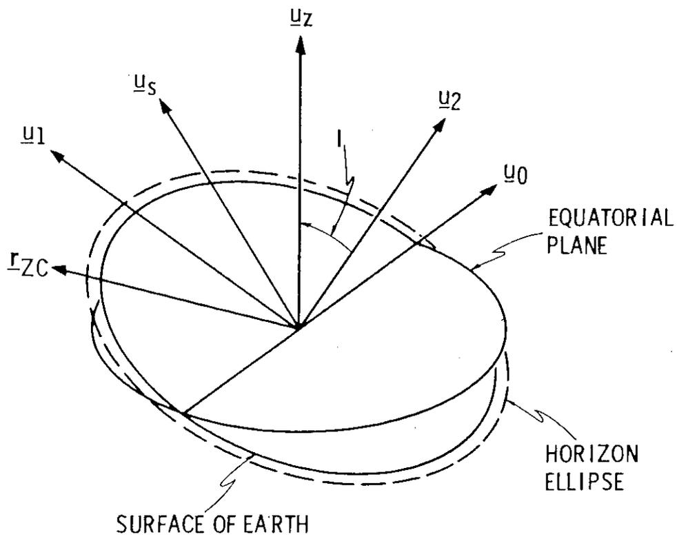
Figure 2.6-1 Definition of Horizon Coordinate System
