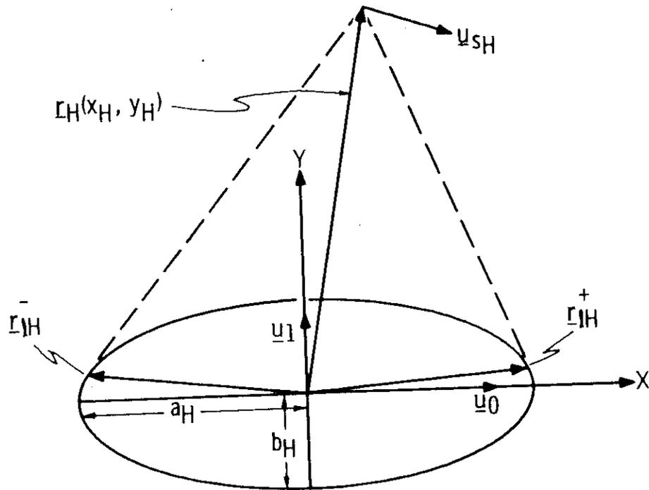
Figure 2.6-2 Geometry of Star-Horizon Measurement
